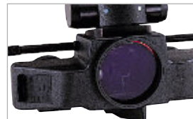
Separate fine-tuning of the illumination beam \pm 4^\circ in addition to synchronized convergence and parallax adjustment.
